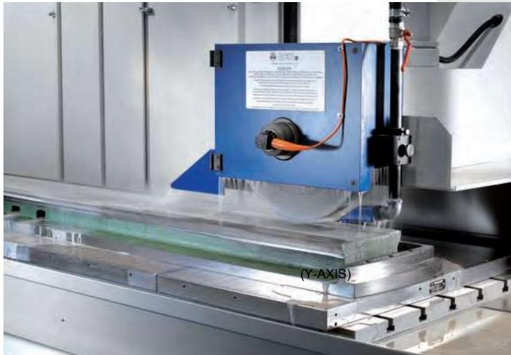
The use of quality perlitic cast iron is employed for the production of all major components of our SR-CNC plane surface grinders.
